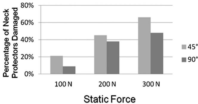
**FIGURE 4.** Percentage of neck guards damaged for each test condition neck guard, a risk that increased force and the 45-degree angle.
