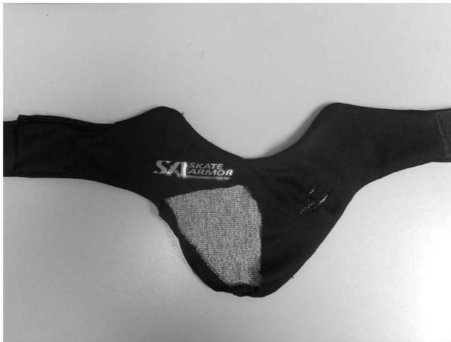
**FIGURE 5.** A skate armor neck guard with the spectra fibers showing. Spectra fibers have higher tensile strength and modulus of elasticity than Kevlar fibers.
