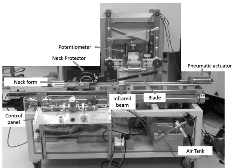
**FIGURE 1.** Picture of the laceration machine. The control panel controls the firing of the laceration machine and has 2 buttons for the “hold and fire” system.
