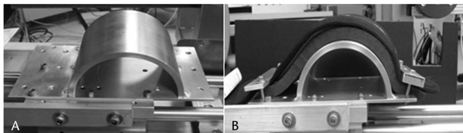
**FIGURE 2.** A, The aluminum neck form has a radius of 57.5 mm and 5 mm thick wall. B, The foam was placed directly onto the neck form, and the neck guard was tightly fitted above the foam.
