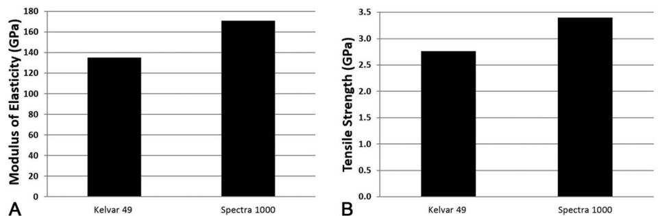
**FIGURE 6.** Mechanical properties of the Spectra fibers and Kevlar (A). Spectra fibers had a modulus of elasticity and tensile strength 27% and 23% higher than Kevlar (B).
